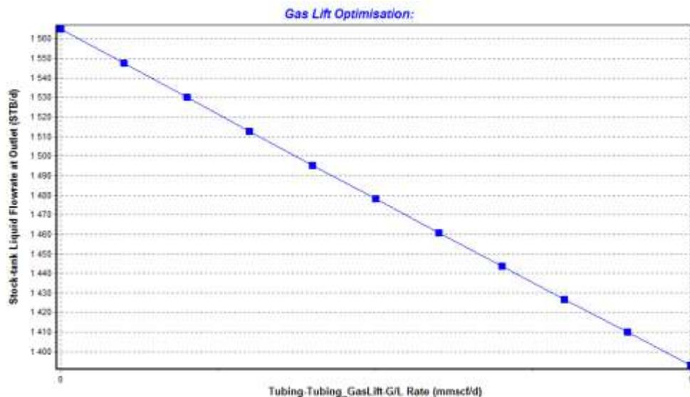
Figure 1 – Flowrate drop with increased gas-oil ratio in horizontal pipe
