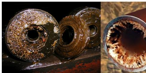
Figure 1 – Salt deposits at pipelines
