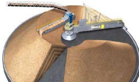
Fig. 2. Circular blending bed with stacker and reclaimer
