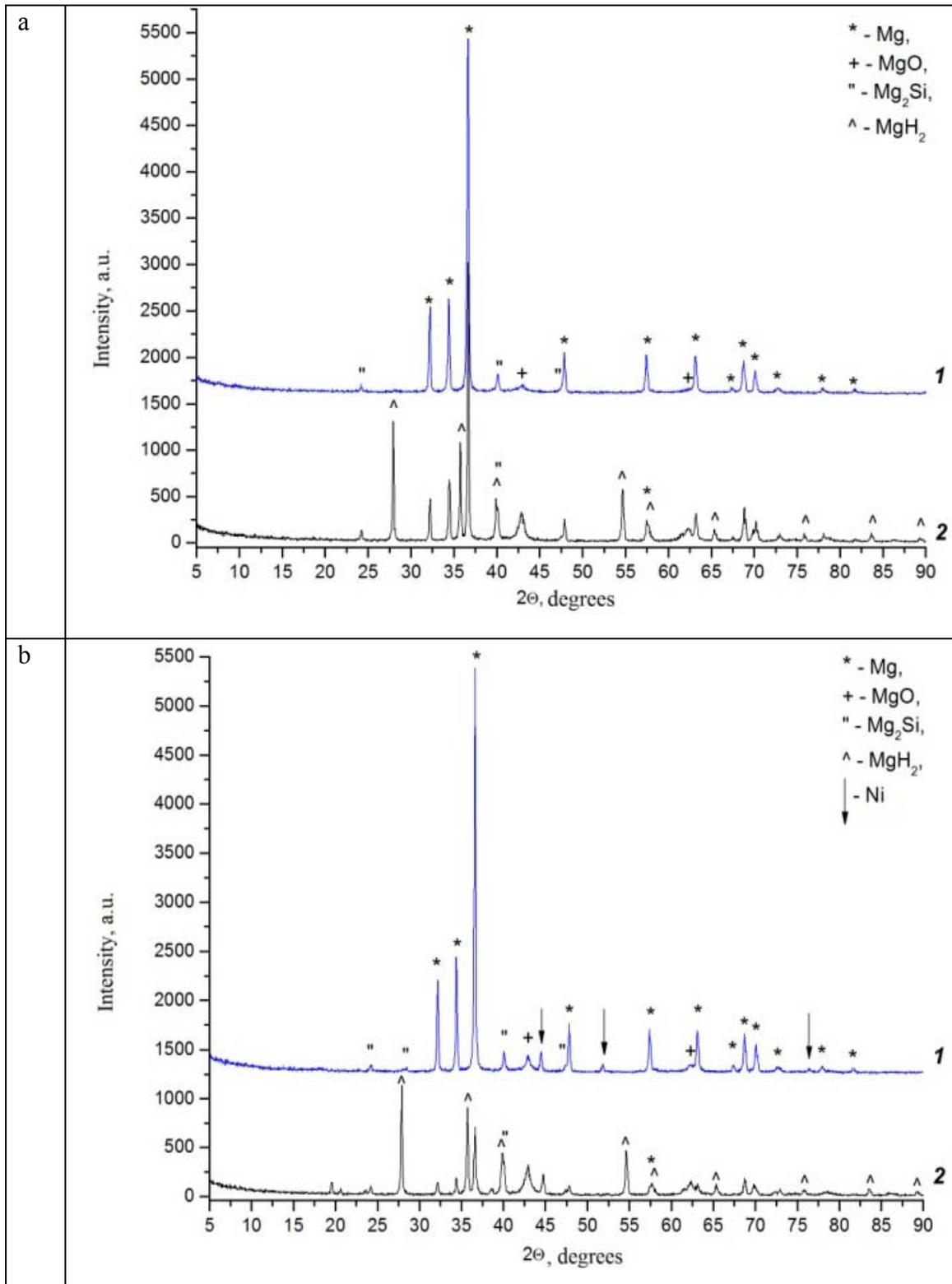
Fig.3. X-ray diffraction diagrams of the samples before (1) and after hydrogenation under pressure (2): a) - sample 1, b) - sample 2;
