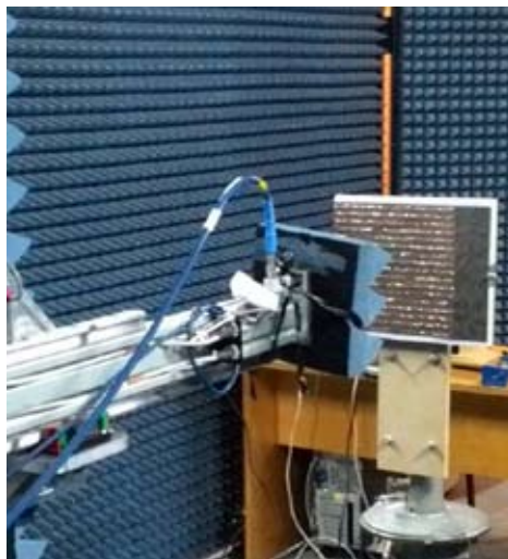
Fig. 2. Photograph of substrate integrated waveguide slot antenna array in anechoic chamber
