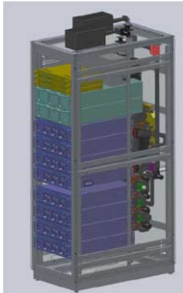
Fig. 6. 4 kW GaN X-Band PowerMAX n+1 Redundant High Power Amplifier System
