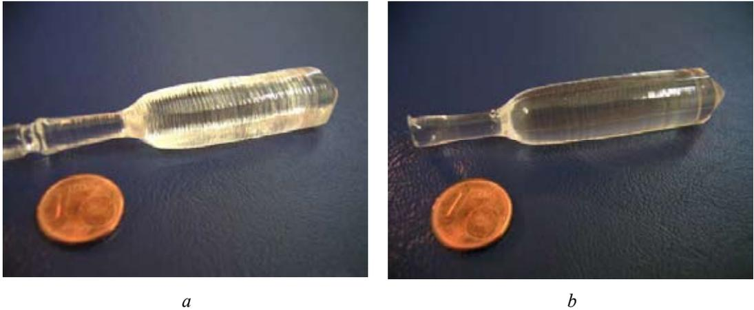
Fig. 2. Crystals grown in b-direction (a) and in c-direction (b)
