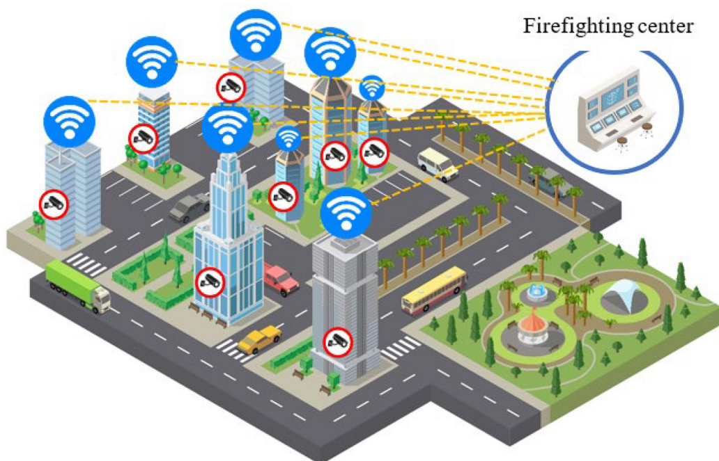
Fig. 3. Depicts the communication network connecting the monitoring stations to the fire control center
