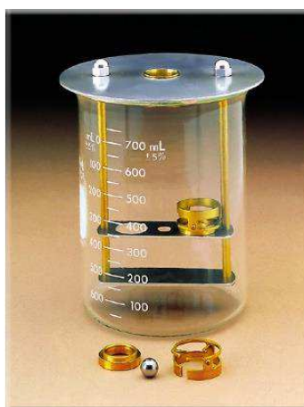
Figure 6 – Softening point apparatus [27]
