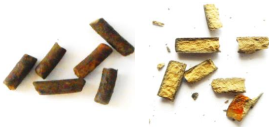
Fig.1. Appearance and inner part of the reforming catalyst after several cycles of regeneration
