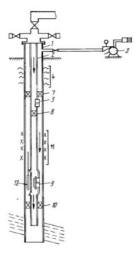
**Figure 1.** Packers installation diagram (packers marked with crosses 7,8,10).
