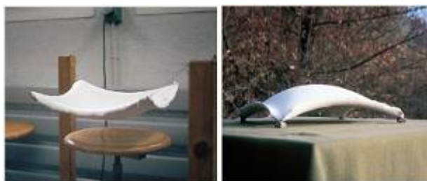
Figure 3. The hanging membrane, once hardened, is inverted to create a shell form in pure compression. Extracted from [13].
