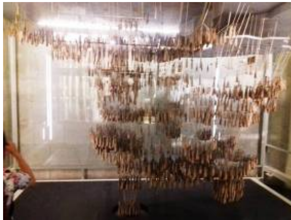
Figure 2. Reproduction of Gaudí's hanging model for the crypt of Colònia Güell, Barcelona.
