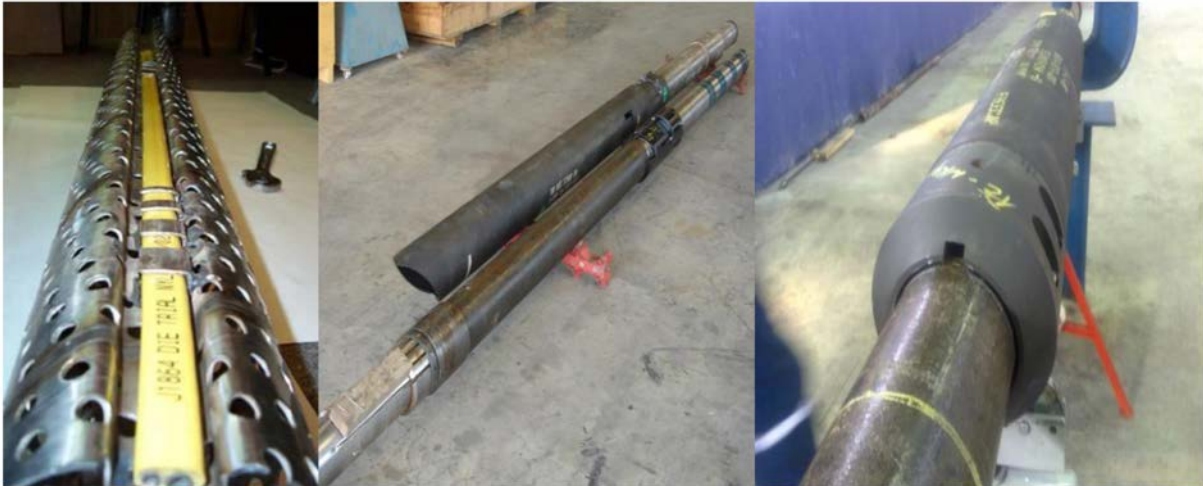
Figure 13—Sand screen with fiber optic cable in a flat braid; system stinger and receiver; swellable packers with wired channels
