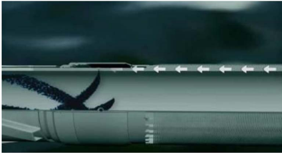
Figure 5—Nozzle based inflow control devices.
