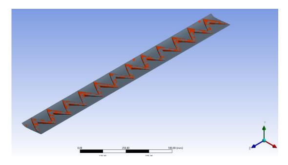
Figure 2 - Result of the blade topology optimization
