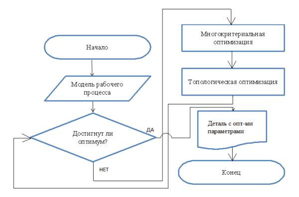
Figure 3 - Consistency of detail geometry optimization tools application with predetermined topology
