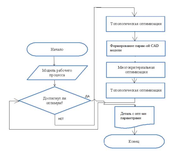
Figure 4 - The algorithm for generating the geometry in a given domain with followed multiobjective optimization
