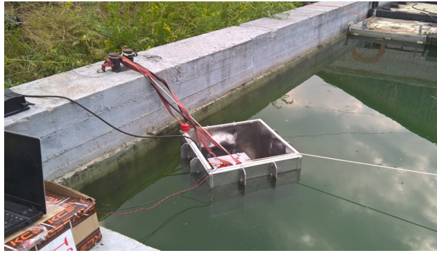
Fig. 2. EMSS model lowered in a test water tank
