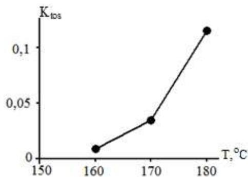
**Figure 9.** Dependence of the coefficient of thermo-oxidative stability on the test temperature of a partially synthetic Mazda Original 10W-40SL/CF engine oil (test time 16 hours).
