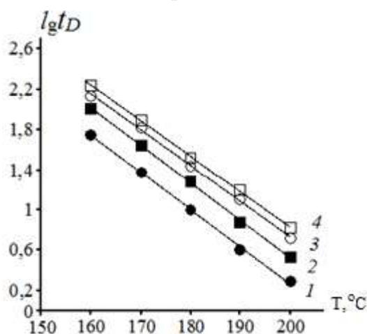
**Figure 2.** Dependence of the decimal logarithm of the time to reach the optical density on the test temperature of a partially synthetic Mazda Original 10W-40 SL/CF motor oil: 1 -  $D = 0.05$ ; 2 -  $D = 0.1$ ; 3 -  $D = 0.2$ ; 4 -  $D = 0.3$ .
