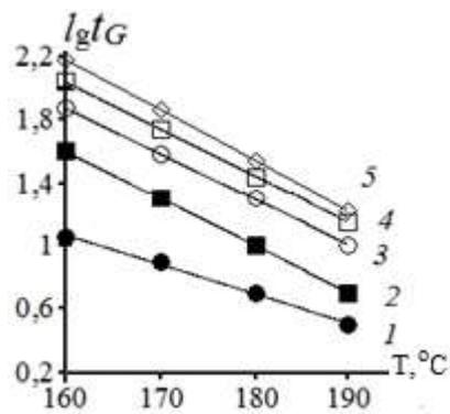
**Figure 5.** Dependence of the decimal logarithm of the time to achieve evaporation on the temperature of testing partially Mazda Original 10W-40 SL/CF synthetic engine oil: 1 - G = 1 g; 2 - G = 2 g; 3 - G = 3 g; 4 - G = 4 g; 5 - G = 5 g.
