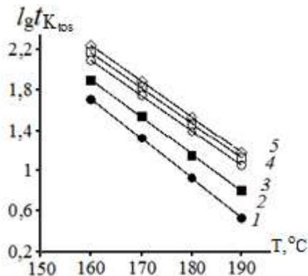
**Figure 8.** Dependence of the decimal logarithm of the time to achieve the coefficient of thermo-oxidative stability on the test temperature of a partially synthetic Mazda Original engine oil: 1 -  $K_{tos} = 0.05$ ; 2 -  $K_{tos} = 0.1$ ; 3 -  $K_{tos} = 0.2$ ; 4 -  $K_{tos} = 0.3$ ; 5 -  $K_{tos} = 0.4$ .
