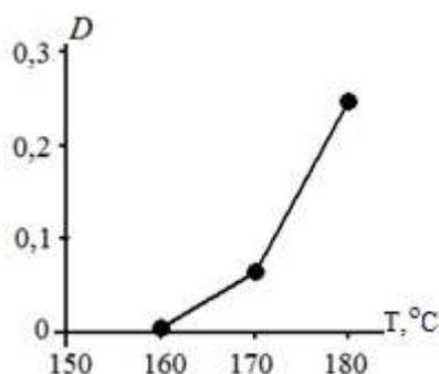
**Figure 3.** Dependence of optical density on the test temperature of a partially synthetic Mazda Original 10W-40 SL/CF engine oil (test time 32 hours).
