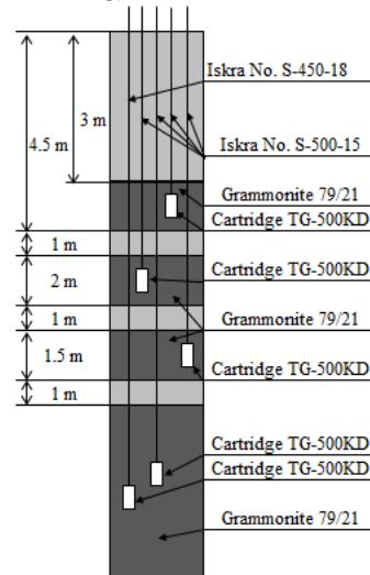
**Figure 5.** Combined (dispersed) composition of the blasthole charge for hard blasted rocks (based on measurements of the load) ("Iskra" No. S-450-18 — 1 unit, "Iskra" No. S-500-15 — 4 units, Ammonite No. 6ZhV — 24 kg, cartridge of 2.85 kg, Grammonite 79/21 — 760 kg)
