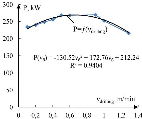
Figure 1. Empirical relation  $P=f(v_{\text{drilling}})$  for DM-H drilling rig
