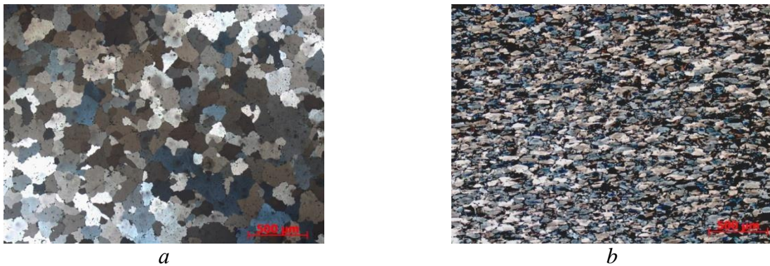
Fig. 5. Microstructure of metal in polarized light, \times 50 : a – cast state; b – deformed state
