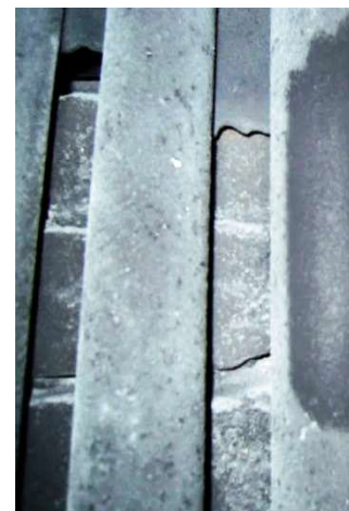
Figure 1. The view of surface of screen tubes: a) before the application of additive; b) after the application of the additive
