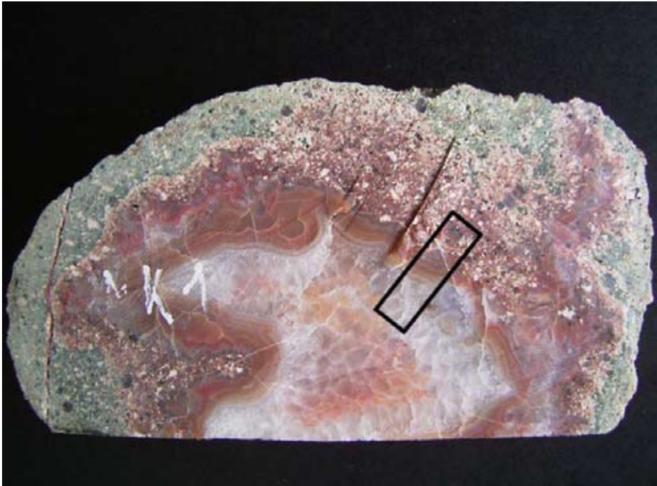
Fig. 2. Selected agate from Nowy Kościół (Poland) for detailed LA-ICP-MS investigations; the rectangle represents the prepared area for the trace-element profile
