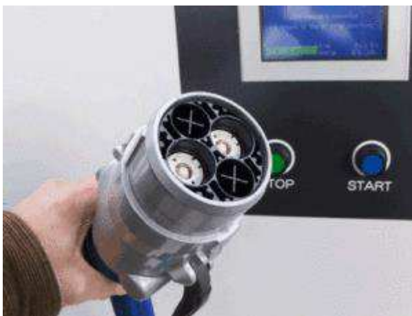
Рисунок 9 – Combined Charging System
