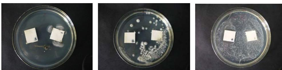
Fig. 3. Growth of *A. pullulans* (left), *P. phoeniceum* (middle), and *S. aureus* (right) cultures on pasteboard samples modified by silver nanoparticles (note, the white spots correspond to microbial colonies). Sample #1 is a control sample, i.e., it was covered with nonmodified paint; sample #2 was covered with the paint modified by silver nanoparticles at a density of 0.8 µg/cm<sup>2</sup>
