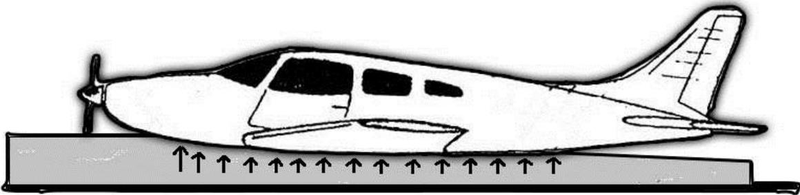
Figure 4 - Scheme of aircraft emergency landing on a polymer mat
