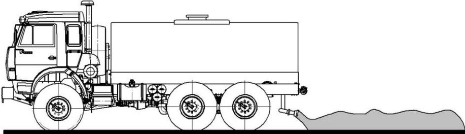
Figure 3 – Foam generating unit PGU-M spreads polymer fireproof material
