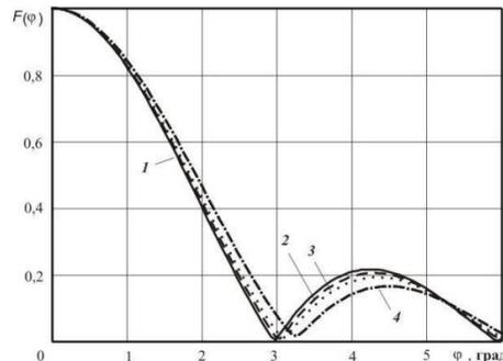
Figure 1 – the change of the antenna RP due to the deformation produced by vibrations.
