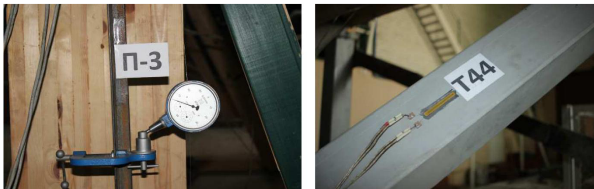
Figure 5. An Aistov 6-ПАО-0.01 deflectometer and a resistance strain gauge
