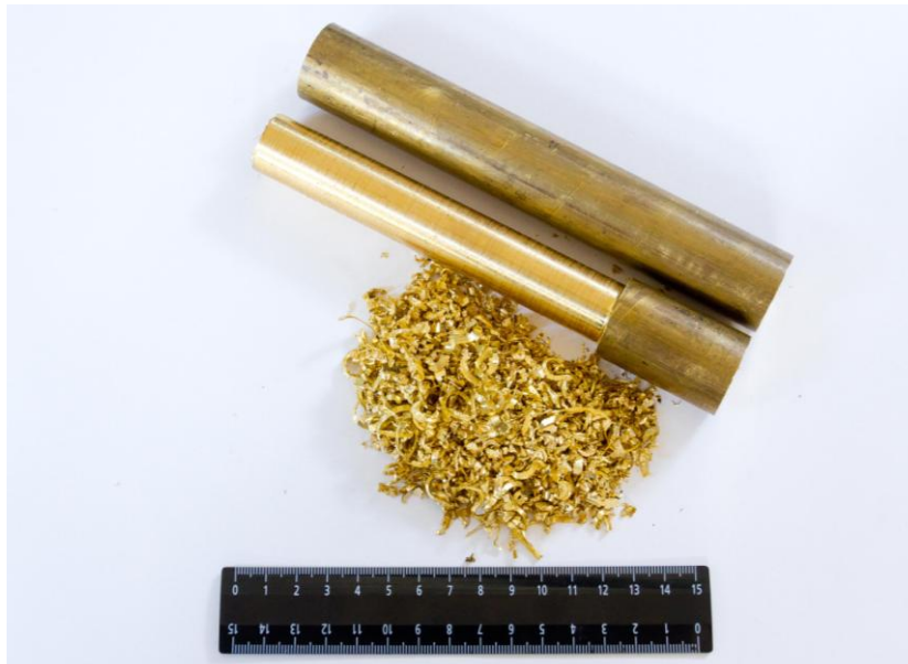
Picture 1 – Type of the bar and shaving formed after turning
