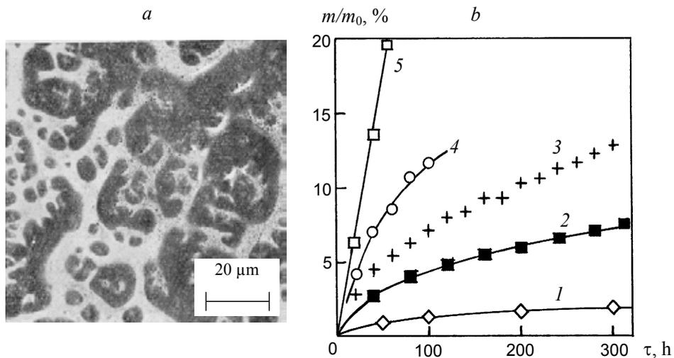
Fig. 4. Microstructure (a) of the film surface and kinetic curves (b) and evaporation of volatile CI G-2 from the film: CI concentration: 1+3 – 0.09 wt %; 4 – 1.4 wt %; 5 – G-2 in its original state. Temperature 25 °C (1, 4, 5), 50 °C (2), and 60 °C (3)
