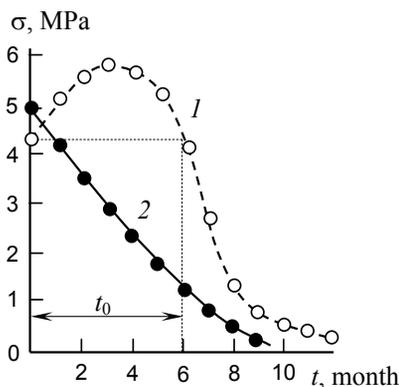
Fig. 7. Ultimate tensile strength of starch-filled (20 wt %) polyethylene films vs. exposure time in soil: 1 и 2 – non-electret and electret films;  $t_0$  – biodestruction incubation period of non-electret film
