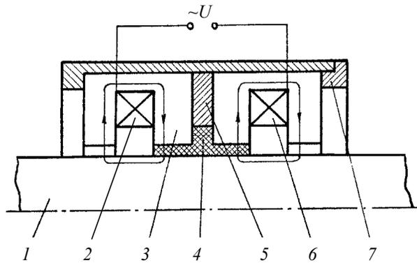
Fig. 6. Induction liquid-metal liner: 1 – ferromagnetic shaft; 2, 6 – energizing coils of electromagnets; 3 – magnetic circuit; 4 – T-shaped porous ring with liquid-metal filler; 5 – diamagnetic dividing bushing; 7 – seal unit case
