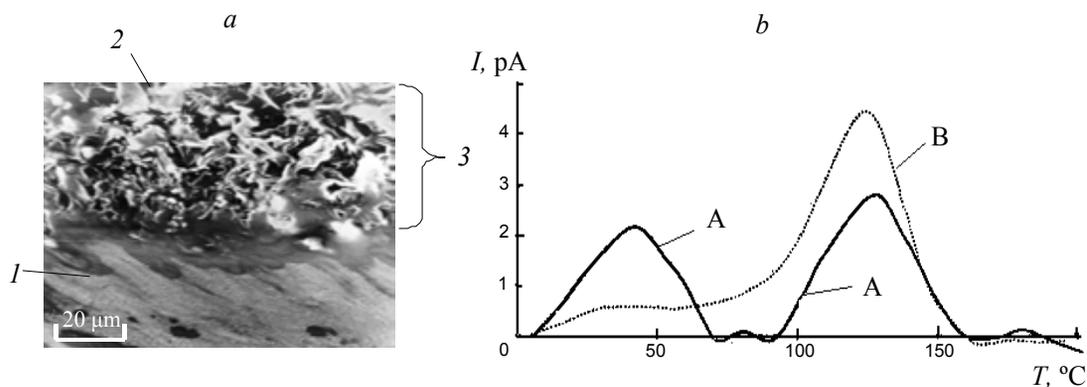
Fig. 5. Cross section (a) and TSC spectra (b) of UHMWPE cartilage: 1 – initial UHMWPE structure; 2 – friction surface; 3 – microporous layer. A – initial sample; B – after friction in synovia ( $p = 2$  MPa,  $v = 0.1$  m/s)
