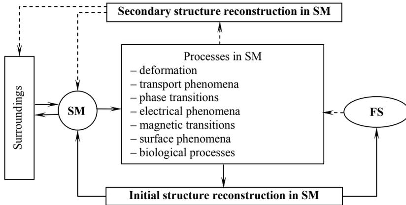
Fig. 1. Diagram of bonds via which the structure of smart material (SM) and surroundings interact with assistance of feedback system (FS). The continuous lines correspond to the primary reconstruction and the dashed lines correspond to secondary reconstruction of SM structure
