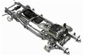
In a body-on-frame vehicle, the vertical surfaces are simply bolted to the frame.
