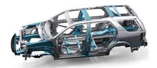
Though a unibody vehicle may have frame rails, those rails are tied to the vertical surfaces of the body to increase strength. In some cases, vehicles are a combination of both construction techniques.
