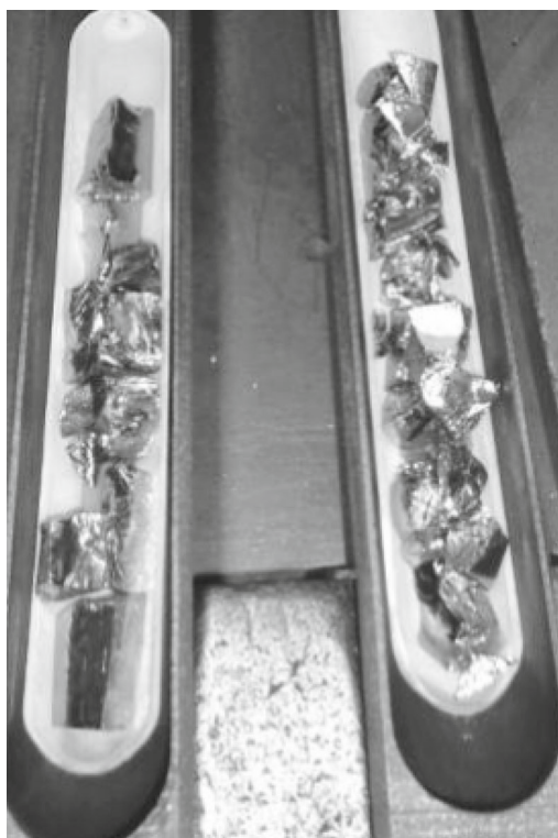
Fig. 5. Test containers with germanium charges.
