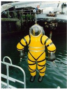
The Hardsuit is the world's most advanced Atmospheric Diving Suit (ADS). It is produced by Ceanic Corporation. The Hardsuit is the product of improvements to existing ADS technology and an innovation breakthrough in a rotary joint development that allows to do low friction movements under an extremely high pressure. This innovative technology enables trained operators to work in water depths up to 305 meters.
