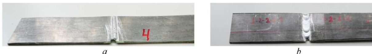
Fig. 5. Type of strip from the side of the weld (a) and back side (b)
